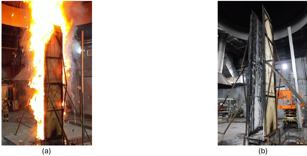
Figure 7-20: FlexPV MP (Test #9) photographs: (a) peak HRR instant, and (b) post-test damage.
