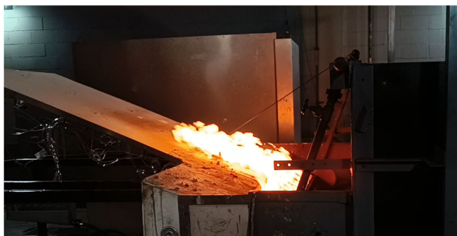
(a) ASTM E108 - roof covers (photo shows the exposure fire to 4 ft long gypsum board)
