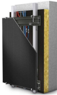
(b) BIPV cavity-wall façade with components cutout
